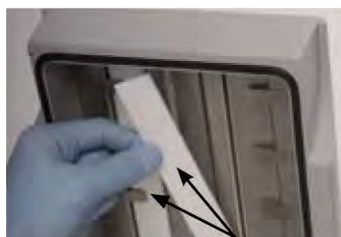
2. Insert two Humidity Control Cards into the lid and saturate with water.
